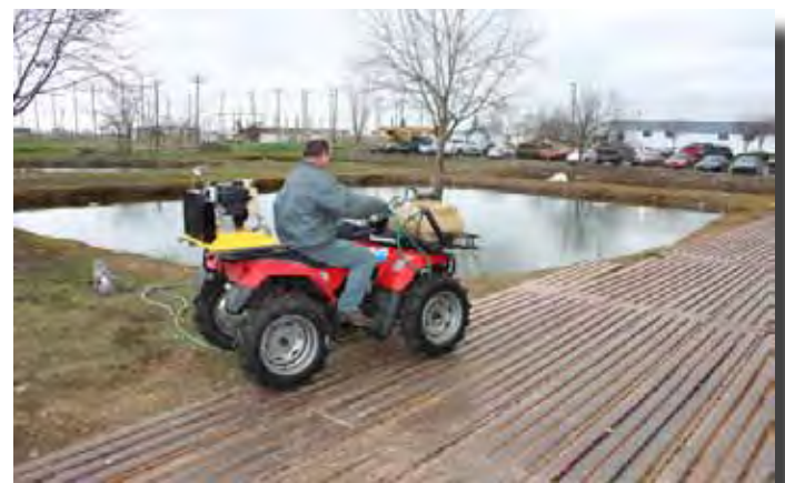
ATV Mounted with fogger and power sprayer
